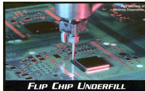
Flip Chip Requires Underfill
